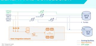
This project can reduce unnecessary heat loss. This resulted in a reduction in fuel consumption by 5,626 tons per year and TOP's high-sulfur LR consumption by 450 tons per month. The company also benefited from energy savings and feed efficiency improvements. LR was 338 million baht per year.
